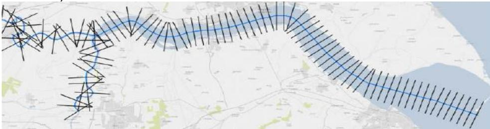
**Figure 4.** Automatic positioning of sections in the Humber Estuary.
